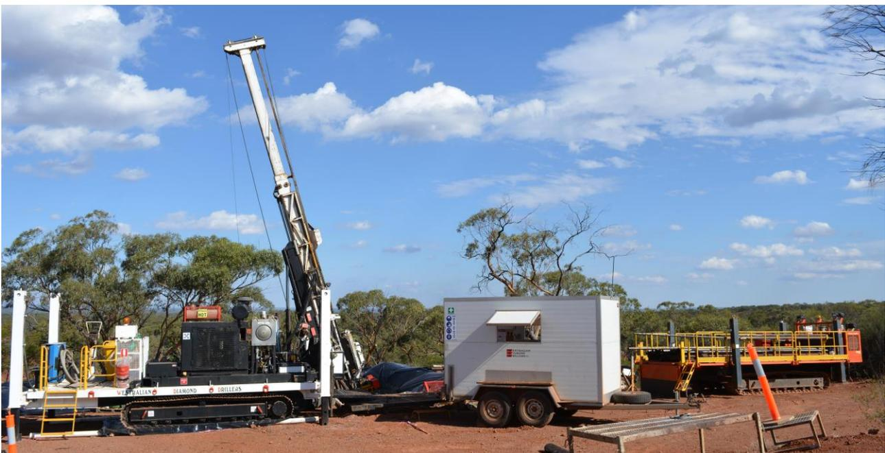
**FIGURE 4 – DIAMOND RIG DRILLING AT ROTHSAY**
